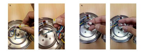
5. You should now be able to remove the receiver and reverse the process to install the replacement.
