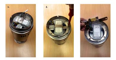
3. Identify the large square connector block which links the remote receiver to the ceiling fan motor. Unclip and separate the block
